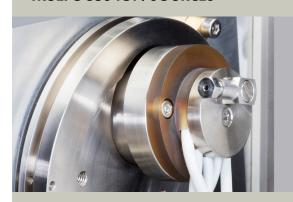
Fischione's history of innovation continues with the introduction of the next generation of ion source technology. Our patented TrueFocus ion sources are now optimized to perform at near 100% ionization efficiency – the result is a highly efficient ion source that maintains a consistent beam current. This technology is built into the Model 1061 SEM Mill.
