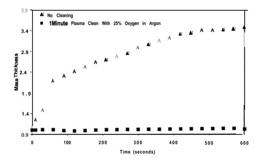
Figure 5. Variation of specimen mass thickness with time before and after plasma cleaning for silicon.
