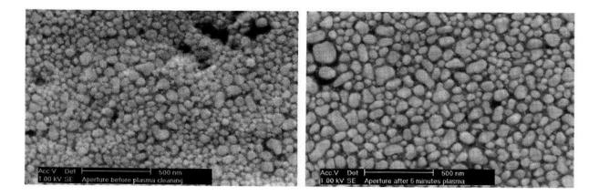
**Figure** 6. SEM micrographs of gold islands on carbon taken a) before and b) after plasma cleaning of the 30 µm SEM objective aperture.
