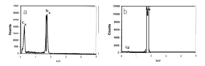
Figure 3. EDS spectra of silicon taken a) before and b) after two minutes of plasma cleaning.
